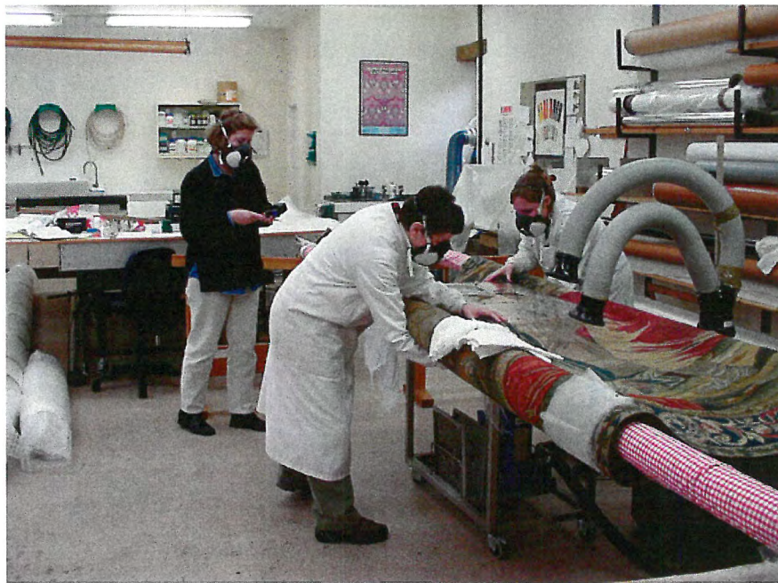
Fig 3 Taking air samples using a Drager Tube system while work in progress on the Ham House tapestry.
