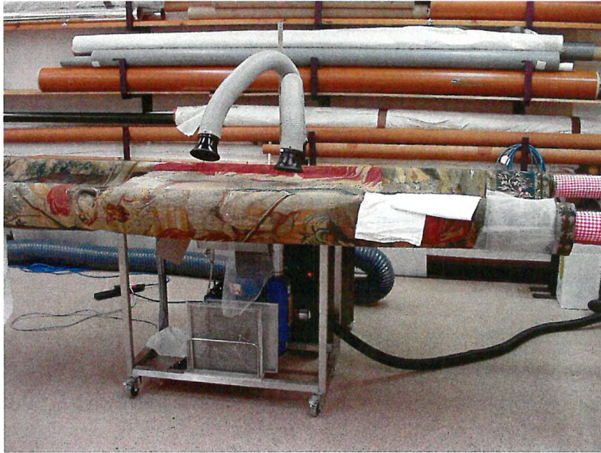
Fig 2 Set up for use of solvents to remove adhesive on the Ham House tapestry.
