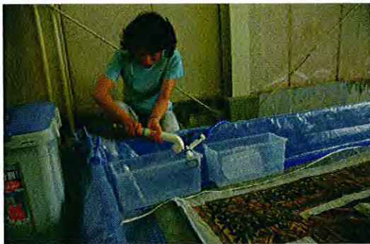
Fig.4 The water was filtered through charcoal filter installed in the showerheads to remove chlorine. The filtered water flowed into the bath from the container where the temperature was controlled at 30°C.
