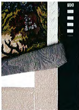
Fig. 3: A model of a wall covering attached to a wooden support frame by staples. The wall covering here is Tyvek. The centimetre gauge indicates the distance between the staples.
