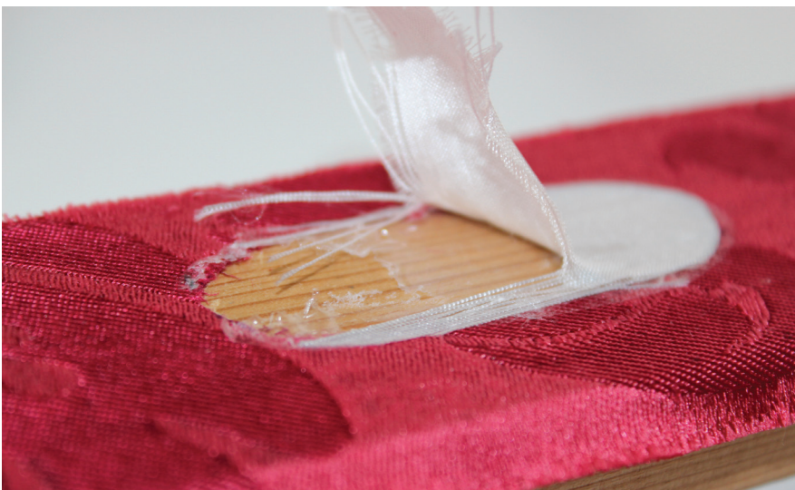
Fig. 19 Unsuccessful heat reversal of Beva® 371 film.
