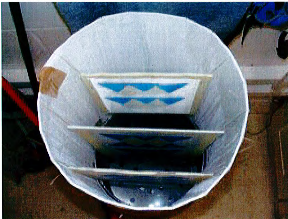
Fig. 6. Burshaw® water boiler modified into a steamer.
