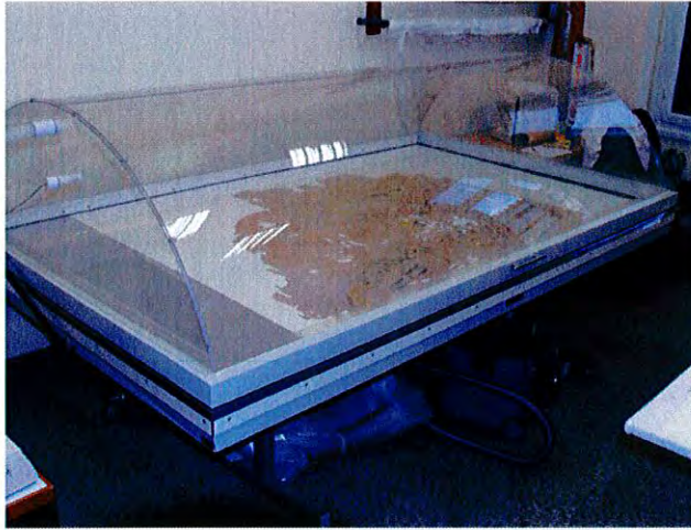
Fig. 8. During humidification and flattening of he object on a suction table with dome.
