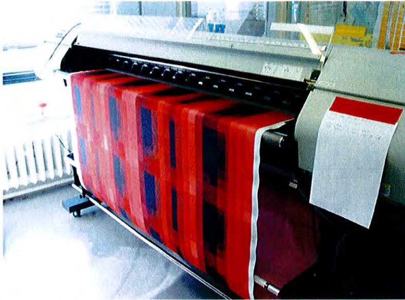
Fig. 1. Mimaki TX 1600 Wide Format Digital Printer in use at the Royal College of Art.
