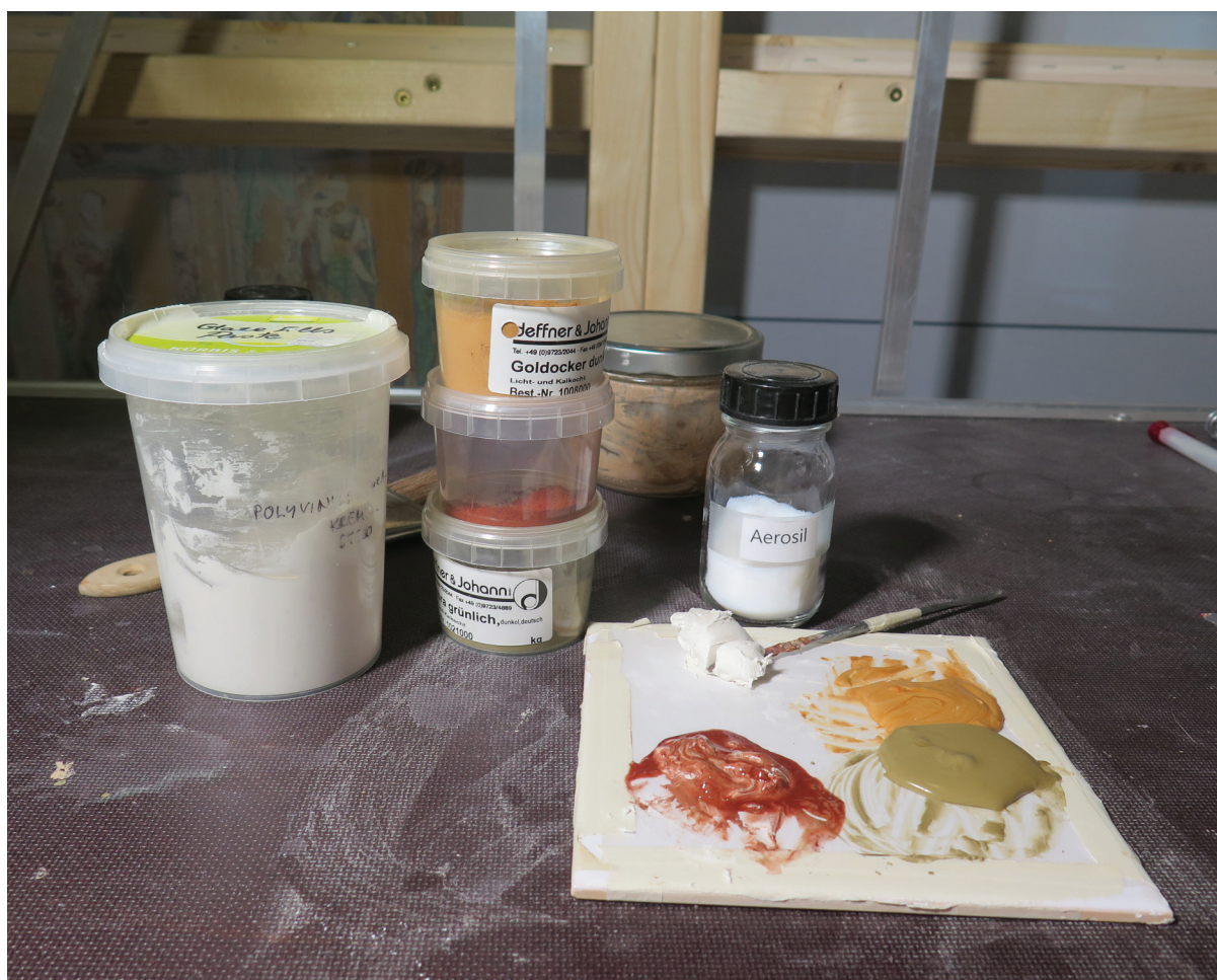
Figure 6. Preparation of fills with polyvinyl butyral, inorganic bulking agents, and dry powder pigments
