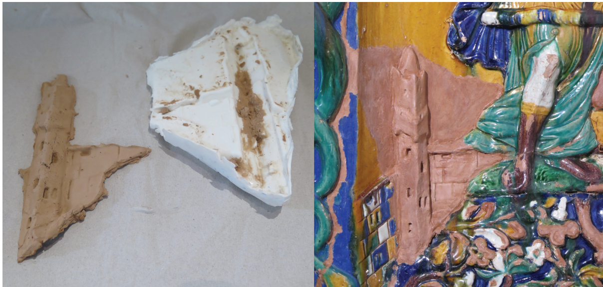
Figure 9. Area of reconstructed tile with the silicone mould made from the original fragment found in the archive (right), and the cast-in coloured polyvinyl butyral putty fill (left)
