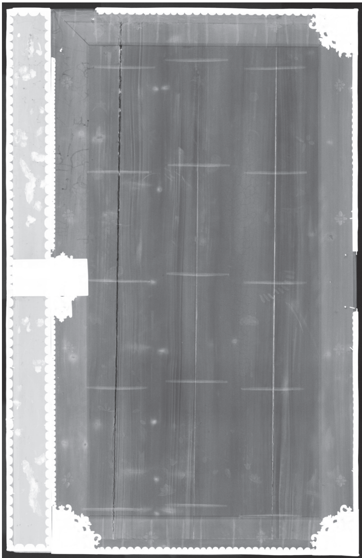
Fig. 2: X-Ray right front doors. Four vertical wooden planks joined with bamboo dowels compose every lacquer panel. On the top and on the bottom two planks close the structure, secured with 13-15 bamboo dowels.
