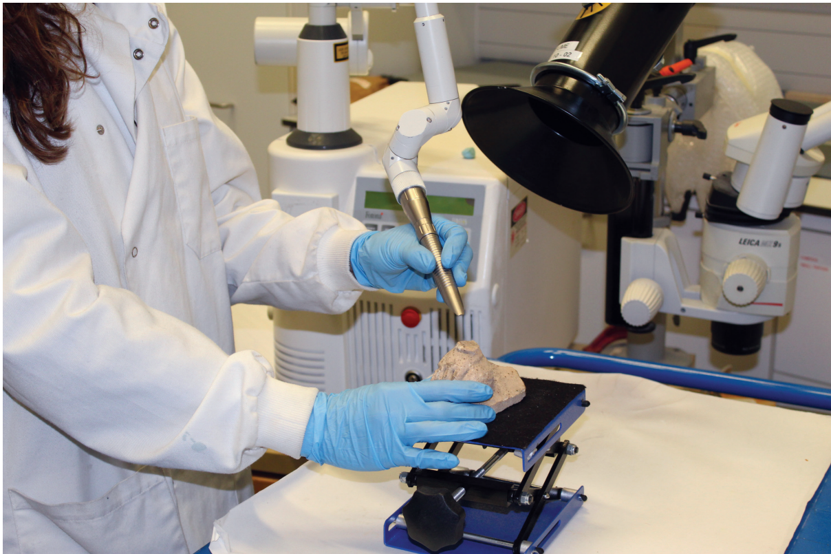
Figure 5. Er:YAG laser at the BM during treatment · Copyright of the Trustees of the British Museum
