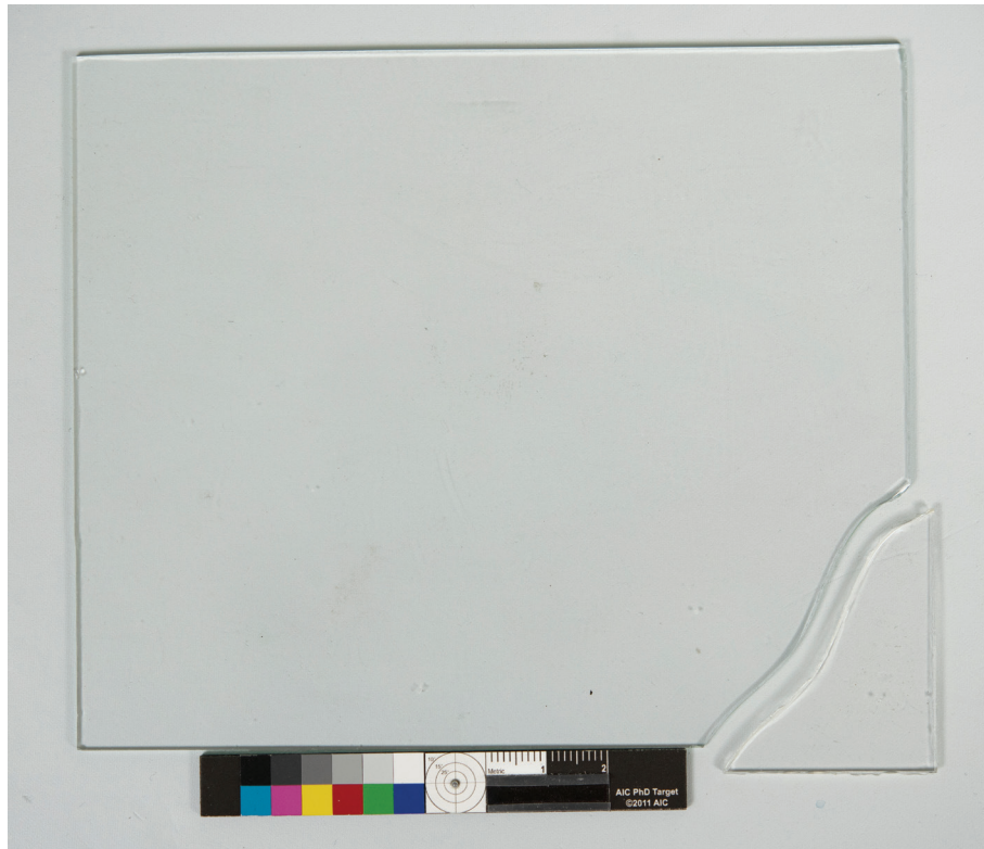
Figure 2. Finished uncoloured PARALOID B-72 thermocast before adhering into a lacuna at the corner of a piece of sheet glass
