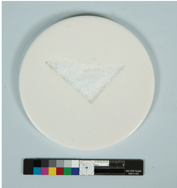
Figure 1. Siliconen Culinair platinum-cured, addition silicone rubber mould filled with ground PARALOID B-72
