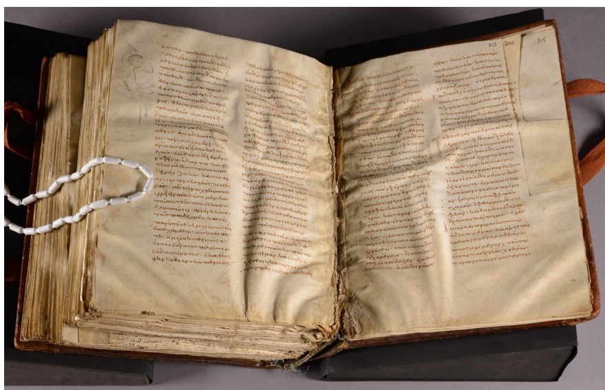
Fig. 5 Cockling and distortion of leaves in the last quarter of the manuscript caused by ingress of water in the past and the use of hot animal glue on the spine.
