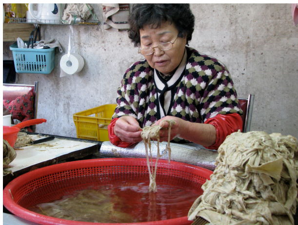
Fig. 6 Picking out impurities. Image copyright Aimee Lee.
