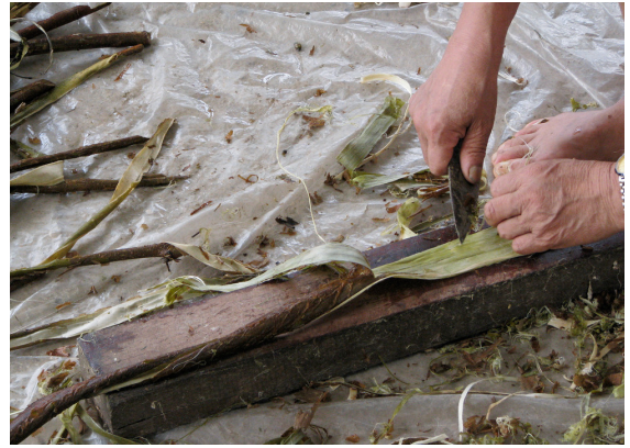
Fig. 4 Removing black and green layers of bark. Image copyright Aimee Lee.
