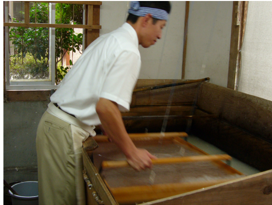
Fig. 10 Japanese nagashizuki sheet formation method by Satoshi Hasegawa. Image copyright Minah Song.
