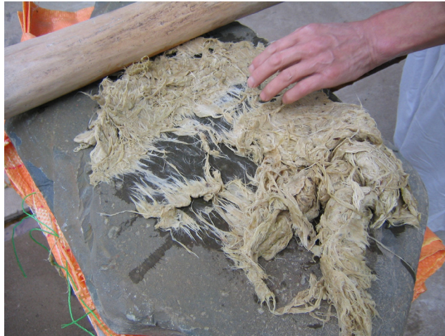
Fig. 7 Beating cooked fibre by hand. Image copyright Bohyung Kim.
