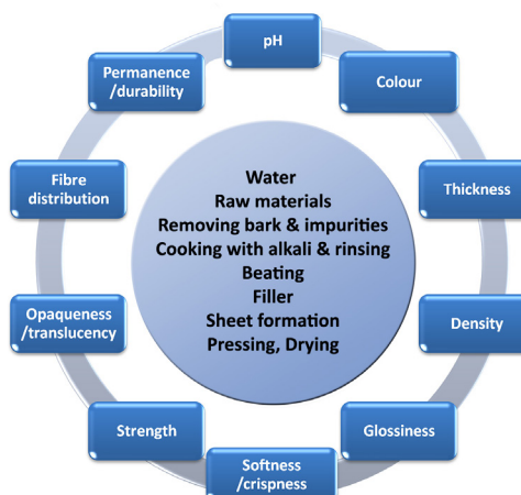
Fig. 14 Key factors in the papermaking process and properties of paper. Image copyright Minah Song.
