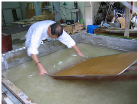
Fig. 9 Korean webaltteugi sheet formation method by Hyunse Shin. Image copyright Bohyung Kim.
