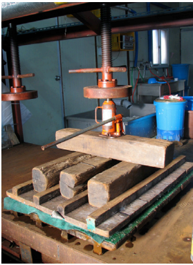
Fig. 11 Pressing the post. Image copyright Aimee Lee.
