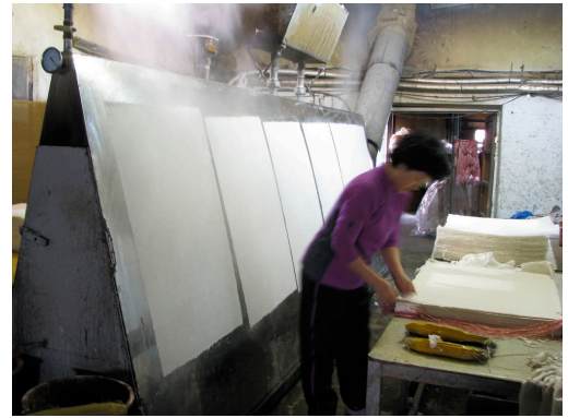
Fig. 13 Drying paper on heated steel dryers. Image copyright Aimee Lee.
