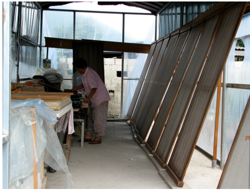
Fig. 12 Drying paper on wooden boards. Image copyright Aimee Lee.
