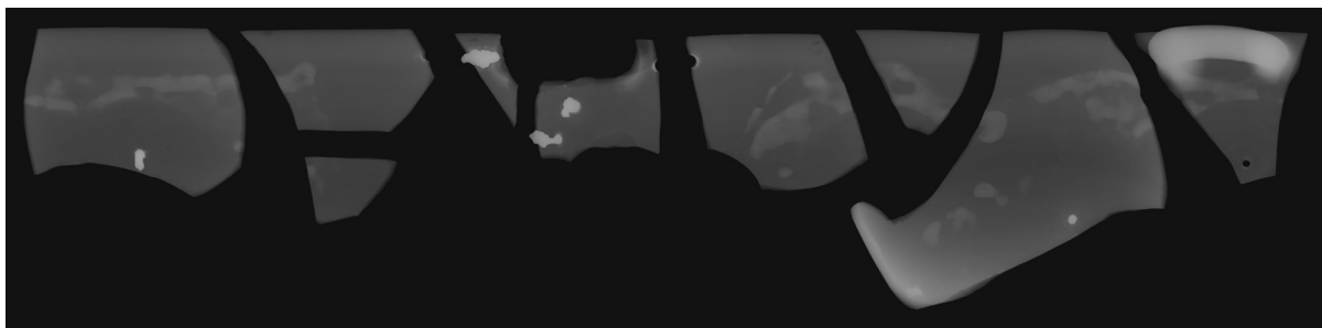
Figure 2. X-radiograph of the disassembled rim sherds of skyphos P.2493/ACP1691b, exposed at 35 kV and 4 mA for 30 seconds
