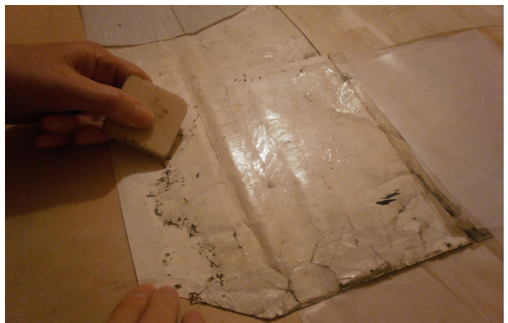
Fig. 6 Adhesive removal with crepe eraser. © The Piper Estate
